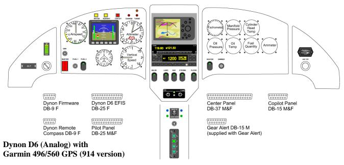
This Wire List includes a guide for connecting seven DB connectors. The optional Harness Installation Kit permits the installer to order the Dynon D6 without a Dynon harness. All the analog instruments are available as a kit from Progressive Aerodyne. The "Pilot Panel" DB-25 (M&F), "Center Panel" DB-37 (M&F) and "Copilot Panel" DB-15 (M&F) connectors are normally mounted on an optional Harness Support Tray.
