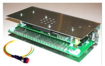
16v. An optional feature can replace a split master switch by removing power to the regulator "C" terminal any time the master switch is turned off. During engine start the SeaRey Power Buss also automatically removes power from the sensitive avionics systems on its six-circuit avionics buss. The SeaRey Harness is pre-wired for the Power Buss. (Please also refer to the Power Buss Installation Manual.)
