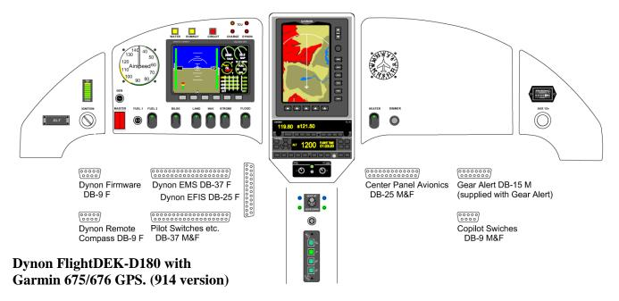
This SeaRey Harness Wire List includes a guide for connecting eight DB connectors behind the panel. The optional Harness Installation Kit contains these connectors and therefore there is no requirement to purchase cables from Dynon for the FlightDEK-D180. The "Pilot Switches" DB-37 (male and female), "Center Panel Avionics DB-25 (male and female) and "Copilot Switches DB-9 (male and female) connectors are normally mounted on an optional Harness Support Tray just ahead of the rudder pedals.
