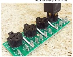
**2090 Gear Position LEDs** These 12v LED kits are appropriately sized for use on the instrument panel and/or center console. The Gear position LED's have an extra wire for use with the ACI gear alert system.
